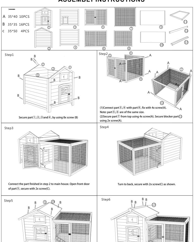
(1)Secure roof part and 0, using 4x screw(B); Attach roof cap part 3, secure with 4x screw(B). (2)Insert metal tray part 1
